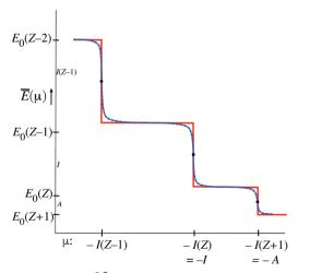
Fig. 4 Step behavior of  $\bar{E}(\bar{N})$  as a function of the parameter  $\mu$  for small T(blue dashes) and in the limit  $T \to 0$  (red lines). For small T the steps are soft. Heavy black dots: values of  $\bar{E}(\mu)$  independent of T; small black dots: values of  $\bar{E}(\mu)$  obtained in the limit  $T \to 0$  only
