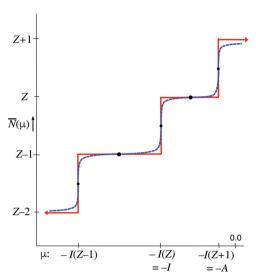
Fig. 3 Steps in the average electron number  $\bar{N}$  as a function of the parameter  $\mu$  in the limit  $T \to 0$ . For T small the steps are soft, see the blue dashed line. Heavy black dots: values of  $\bar{N}(\mu)$  independent of  $T_i$  small black dots: values of  $\bar{N}(\mu)$  obtained in the limit T=0 only.
