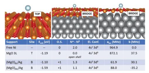
Fig. 6 Ni adatom. Most favourable adsorption mode on MgO 3L (left),  $(MgO)_{BL}/Ag$  (middle) and  $(MgO)_{ML}/Ag$  (right). Adsorption site (T = O top, B = bridge), adsorption energy ( $E_{ads}$ ), formal oxidation state of the adatom (O.S.), number of unpaired electrons ( $N^{\alpha} - N^{\beta}$ ), electron configuration (El. Conf.), and isotropic (a<sub>iso</sub>) and anisotropic (b) hyperfine parameters.
