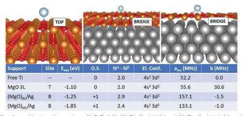
Fig. 1 Ti adatom. Most favourable adsorption mode on MgO 3L (left),  $(MgO)_{BL}/Ag$  (middle) and  $(MgO)_{ML}/Ag$  (right). Adsorption site (T = O top, B = bridge), adsorption energy ( $E_{ads}$ ), formal oxidation state of the adatom (O.S.), number of unpaired electrons ( $N^{\alpha} - N^{\beta}$ ), electron configuration (El. Conf.), and isotropic (a<sub>iso</sub>) and anisotropic (b) hyperfine parameters.
