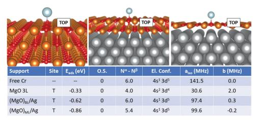
Fig. 2 Cr adatom. Most favourable adsorption mode on MgO 3L (left),  $(MgO)_{BL}/Ag$  (middle) and  $(MgO)_{ML}/Ag$  (right). Adsorption site (T = O top, B = bridge), adsorption energy ( $E_{ads}$ ), formal oxidation state of the adatom (O.S.), number of unpaired electrons ( $N^{\alpha}-N^{\beta}$ ), electron configuration (El. Conf.), and isotropic (a<sub>iso</sub>) and anisotropic (b) hyperfine parameters.
