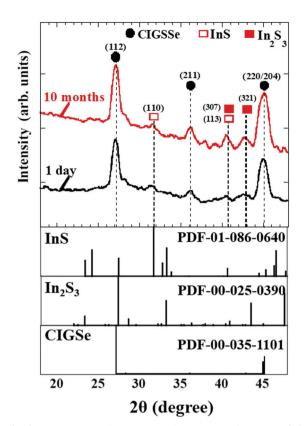
Fig. 18 GIXRD patterns of the near-surface region of the bare CIGSSe thin films (glass/Mo/CIGSSe) for aging times of 1 day, and 10 months. The incident angle of the GIXRD measurement was 0.1°, which corresponds to a corresponding penetration depth of approximately 55 nm into the CIGSSe. Powder diffraction files are denoted as PDF.
