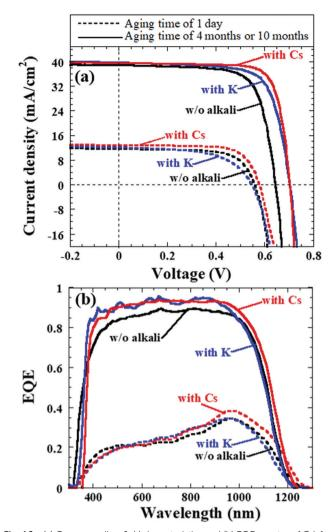
Fig. 16 (a) Corresponding J-V characteristics and (b) EQE spectra of Cd-free and all-dry process CIGSSe solar cells using aged CIGSSe absorbers for aging times of 1 day, as well as 4 months or 10 months, where the absorbers with the alkali (Cs or K) treatment and without (w/o) alkali treatment are utilized.
