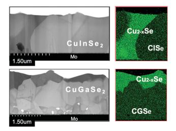
Fig. 12 Cross-sectional STEM images of Cu-rich CISe (upper) and CGSe (lower) samples. The right-hand images show the TEM-EDX mapping of Cu atoms for each sample
