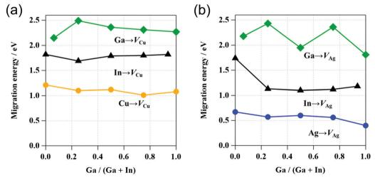
Fig. 8 (a) Activation energies of Cu, In, and Ga migration in Cu-poor Cu( $Ga_xIn_{1-x}$ )Se<sub>2</sub> with CGI  $\sim 15/16$  and (b) those of Ag, In, and Ga migration in Ag-poor Ag( $Ga_xIn_{1-x}$ )Se<sub>2</sub> with [Ag]/([Ga] + [In])  $\sim 15/16$ .
