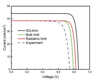
Fig. 19 Current–voltage characteristic curves derived under various calculation conditions or obtained experimentally. The obtained parameters,  $J_{SC}$  and  $V_{OC}$ , are listed in Table 4.
