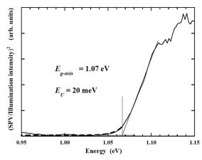
Fig. 22 Relationship between the square of the illumination intensity normalized surface photovoltage (SPV) of the CdS/CIGSSe structure and the photon energy.  $E_{g\text{-min}}$  and  $E_U$  are the minimum of the band gap energy and the Urbach energy of the CIGSSe absorber, respectively. SPV was measured *in situ* using a photo-assisted UHV Kelvin probe force microscope. The dashed fit line results from a fit of the subband gap SPV using the Urbach tails.
