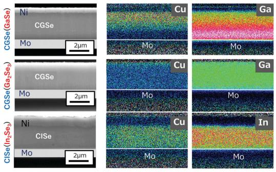
Fig. 11 Cross-sectional SEM images and EDX maps of CGSe and CISe samples. The upper sample was grown from a layered GaSe precursor, the middle using a  $\alpha$ -Ga<sub>2</sub>Se<sub>3</sub> precursor, and the bottom for a  $\gamma$ -In<sub>2</sub>Se<sub>3</sub> precursor. The red dots indicate high intensity signals and the blue dots low intensity signals in the EDX maps. The cross-section of the samples was polished by ion beam etching
