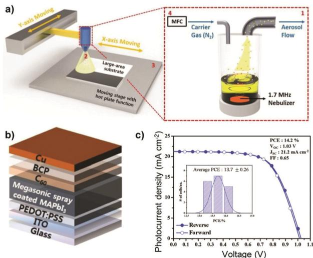
Fig. 4 (a) Schematic representation of the megasonic spray-coating process. (b) Schematic illustration of an inverted planar MAPbI<sub>3</sub> perovskite solar cell fabricated via the megasonic spray-coating system. (c) J-V curves and histogram (inset) of 18 megasonic sprayed perovskite solar cells with a 1 cm<sup>2</sup> active area under one sun illumination. Reproduced with permission.<sup>65</sup> Copyright 2018, John Wiley and Sons.
