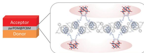
Fig. 1 Stacking layers configuration used to evaluate the effect of **pyrPOM@PCBM** (inset molecular structure) on the performance of the donor (P3HT)/acceptor (PCBM) thin layer OPV device. A bilayer fullerene organization is proposed according to the XRD pattern and the AFM imaging results.
