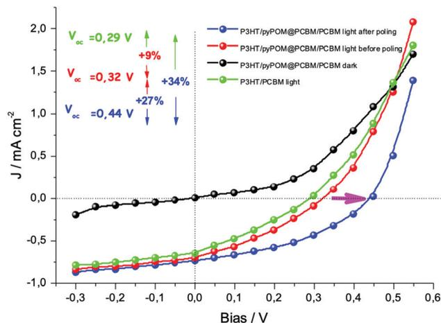
Fig. 7  $J$ - $V$  characteristics recorded for solar devices carried out using as photoactive layers P3HT/PCBM, P3HT/pyrPOM@PCBM//PCBM, P3HT/pyrPOM@PCBM//PCBM after poling (5 V) under 1.5 AM illumination, black curve is referred to the  $J$ - $V$  curve of P3HT/pyrPOM@PCBM//PCBM without the illumination.
