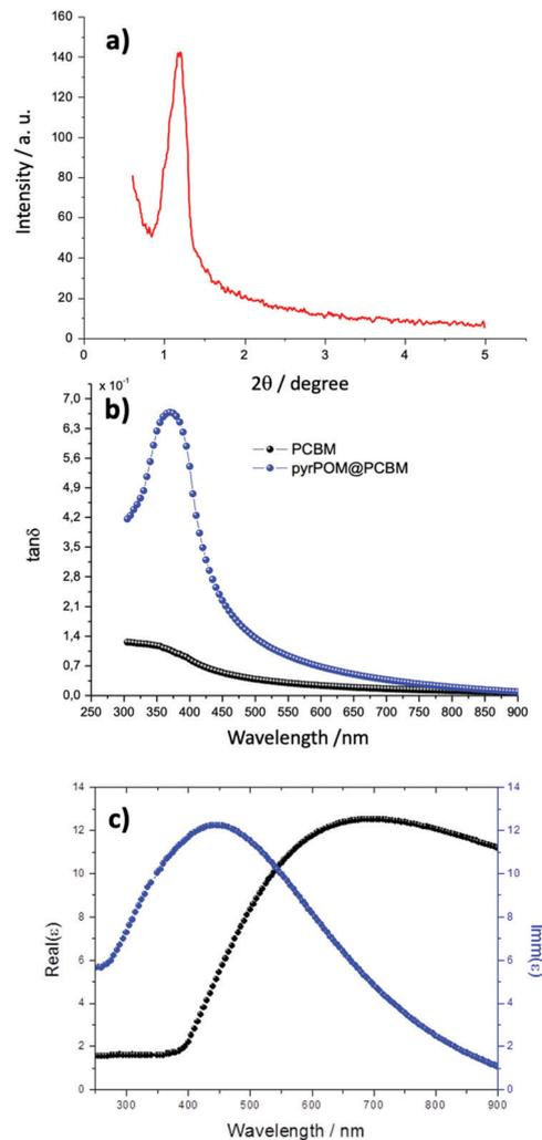
Fig. 4 (a) XRD measurement shows a periodicity of  $(7.6 \pm 0.2)$  nm of the LS pyrPOM@PCBM layer. (b and c) The dielectric loss of pyrPOM@PCBM, dramatically different from that one of PCBM, suggests that an electric dipole is created at the opposite edges of the nanodomains. Increasing the frequency, the dielectric permittivity of pyrPOM@PCBM LS film becomes negligible.
