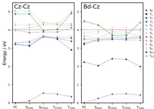
Fig. 5 Energy profiles for singlet and triplet states, including the  $\text{Cz}^-\text{Cz}^+$  and  $\text{Cz}^-\text{Bd}^+$  charge transfer states ( $S_{CT}$  and  $T_{CT}$ ) computed at the critical points for dimer A embedded in the crystal environment using the OEC model.
