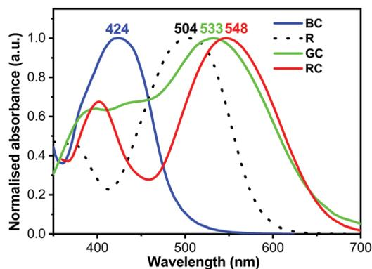
Fig. 3 Normalised absorption spectra of thin films on glass TPA-T-C(O)H (BC), N(Ph-T-CNA-EtHex)<sub>3</sub> (R), N(Ph-2T-DCV-Hex)<sub>3</sub> (GC), and TPA-BTZ-Rh-Et (RC).
