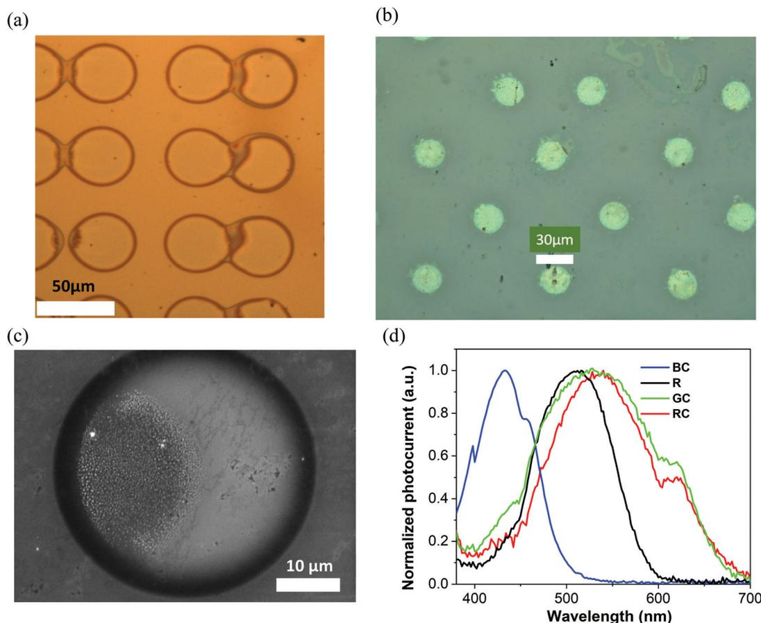
**Fig. 5** Optical microscope image of the (a) TPA-BTZ-Rh-Et pixel array (~42 μm diameter) and (b) N(Ph-T-CNA-EtHex)<sub>3</sub> array (~25 μm diameter), (c) SEM image of a TPA-BTZ-Rh-Et single pixel 42 μm in diameter, at 725 k magnification, and (d) typical normalised photocurrent spectra of inkjet printed small molecule pixels on glass/ITO/ZnO substrates, interfaced with an electrolyte (PBS). Peak position wavelengths are 432 nm (blue), 511 nm ('rods'), 530 nm (green) and 540 nm (red).
