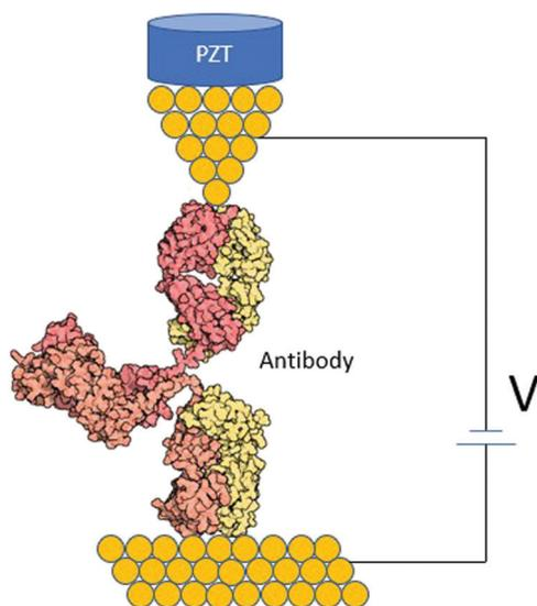
Fig. 7 STM biomolecular break junction formed by an individual antibody between two gold electrodes.
