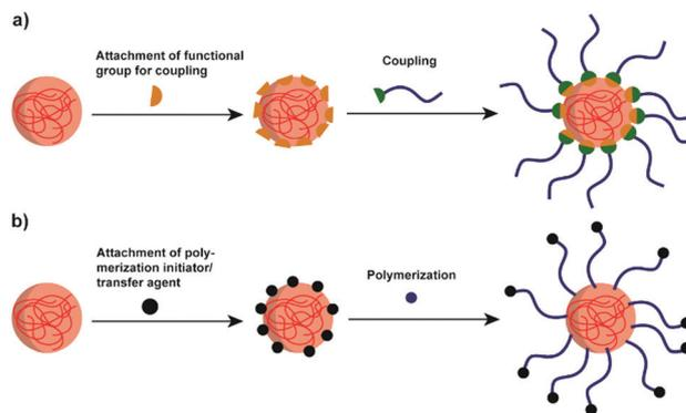
**Scheme 7** Schematic representation of the two grafting approaches. (a) The “grafting to” approach involving the coupling between the polysaccharide NPs and the pre-formed polymer chains (blue line). (b) The “grafting from” approach relying on polymerisation initiated at the NP surface (initiator/transfer agent: black sphere; monomer: blue sphere).
