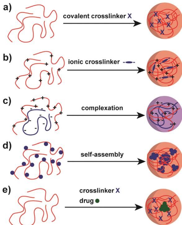
**Scheme 2** Avenues for the preparation of polysaccharide NPs: (a) covalent crosslinking, (b) ionic crosslinking, (c) complexation of oppositely charged polysaccharides, (d) self-assembly of hydrophobically (blue sphere) modified polysaccharides and (e) polysaccharide–drug (green sphere) conjugate.<sup>25</sup>
