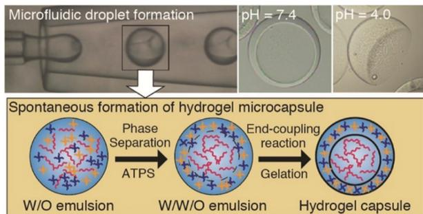
Fig. 8 Formation of PEG/DEX capsules *via* ATPS templating in a microfluidic system. (Reproduced with permission from ref. 204. Copyright American Chemical Society, 2019.)
