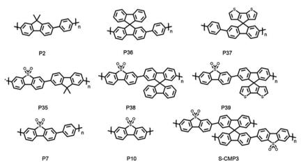
Fig. 1 Structures of the polymer photocatalysts studied here.
