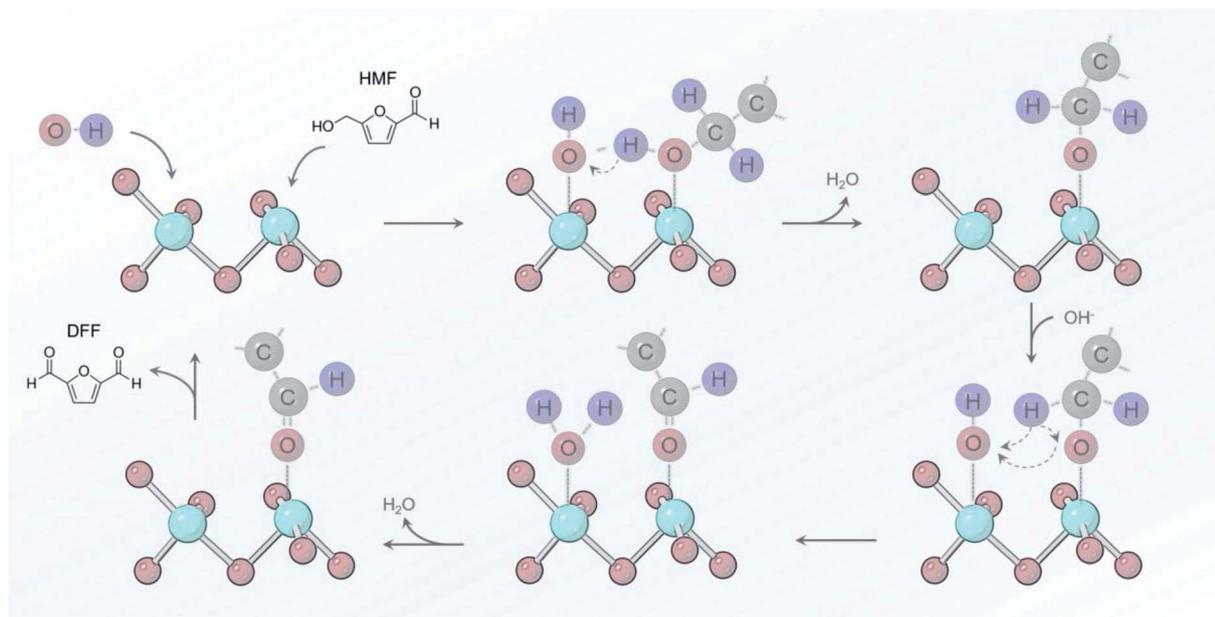
Fig. 7 Reaction pathway proposed for oxidizing the alcohol group of HMF that involves \*OH as a key proton acceptor in pH 12 electrolyte.
