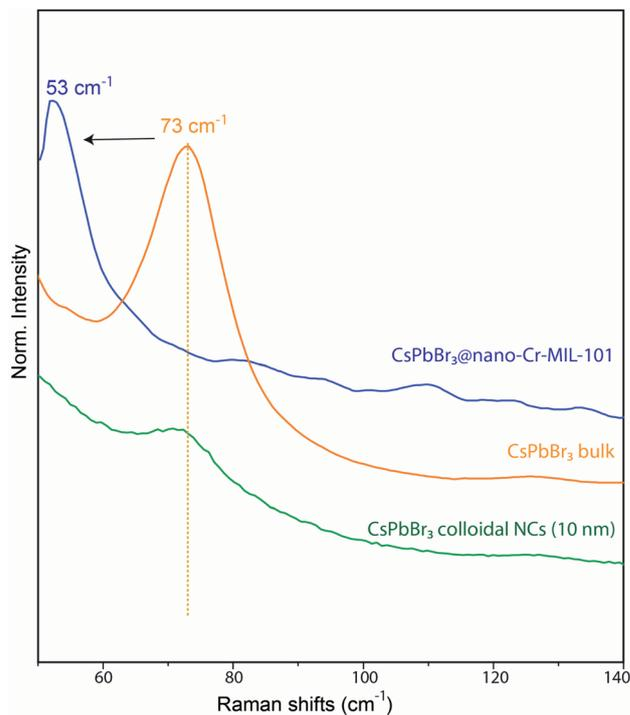
Fig. 3 Comparison between Raman vibrational bands of bulk CsPbBr<sub>3</sub>, CsPbBr<sub>3</sub>@nano-Cr-MIL-101, and colloidal CsPbBr<sub>3</sub> NCs (10 nm).
