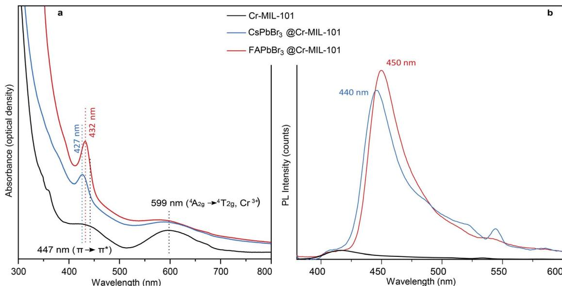
Fig. 4 (a) Absorbance and (b) photoluminescence spectra for nano-Cr-MIL-101, CsPbBr<sub>3</sub>@nano-Cr-MIL-101, and FAPbBr<sub>3</sub>@nano-Cr-MIL-101.
