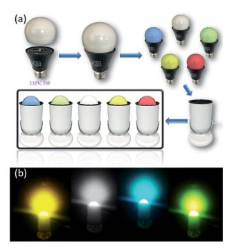
Fig. 6 (a) Schematic showing the assembly of prototype LED lighting devices based on AIO compounds. (b) Illuminating LED light bulbs (110 V, 2 W) coated by selected AIO-type phosphors. Reproduced with permission from ref. 29. Copyright 2020, American Chemical Society.
