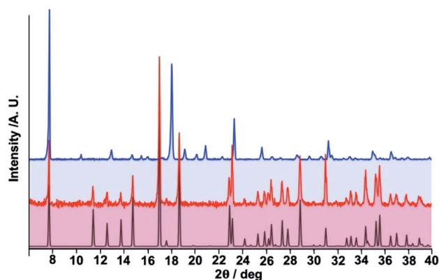
Fig. 6 Comparison of calculated and experimental (black and red lines) powder X-ray diffraction (PXRD) patterns for **1**·PhNO<sub>2</sub> with the experimental PXRD of **1** (blue line).
