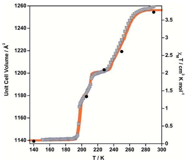
Fig. 2 Comparison of the thermal dependence of  $\chi_{\text{M}}T$  (orange) and unit cell volume (grey dots) for  $1 \cdot \text{PhNO}_2$ . Black filled circles represent the volume–temperature coordinates at which the crystal structure has been solved (15 K LS and HS\* data not shown).
