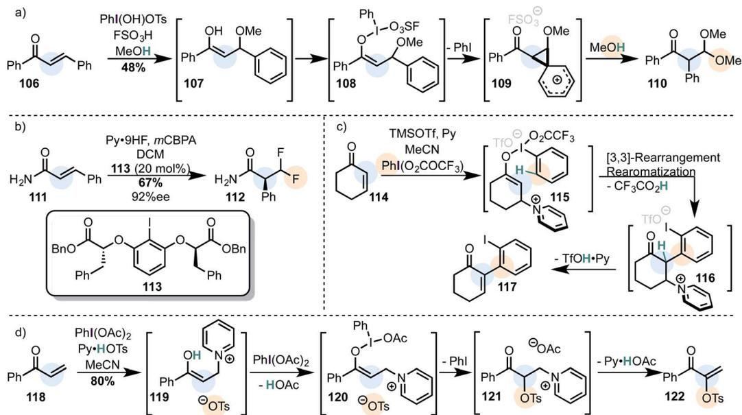
**Scheme 11** Michael acceptors as substrates in 1,4-addition/iodine(III) oxidation tandem reactions. (a) Classical example with methanol as the secondary nucleophile. (b) Catalytic enantioselective difluorination via an iodine(III)-mediated phenyl migration. (c) The 1,4-addition of the bulky pyridine blocks the enolonium species from nucleophilic attack and instead enables an iodonio-Claisen rearrangement. (d) Umpolung of the Morita–Baylis–Hillman reaction.
