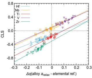
Fig. 7 Calculated core level shifts for all 120 atoms (open markers) in the supercell versus charge transfer compared to elemental references, calculated using the fixed sphere model, i.e. all individual values giving the average  $\Delta q$  (alloy  $a_{\rm relax}$  – elemental ref.) in the last column of Table 1 (also shown here as filled markers).
