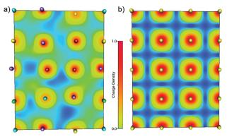
Fig. 4 Electronic density map slices from DFT simulations, for a (100) plane for the  $Hf_{20}Nb_{20}Ti_{20}V_{20}Zr_{20}$  multi-component alloy (a), and a reference bcc metal (b). Different elements indicated by different colour of the spheres: Ti - red, V - purple, Zr - green, Nb - yellow, and Hf - light blue. The colour scale shows the normalized charge density for the respective panel.
