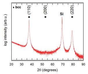
Fig. 8  $\theta/2\theta$  diffractogram of the studied  $Hf_{22}Nb_{19}Ti_{18}V_{19}Zr_{21}$  coating. Diamond markers show positions for the observed bcc phase. The peak at  $2\theta \sim 69^{\circ}$  originates from the Si substrate.
