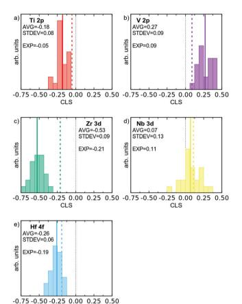
Fig. 6 Histograms of simulated XPS CLS for the 120 atoms of the DFT supercell, divided according to element. Average CLS indicated by a solid line, and experimental value by a dashed coloured line
