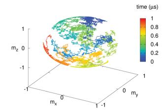
Fig. 1 Magnetisation direction, depicted on the unit sphere, as function of time (colour coded) for an isotropic magnetic nanoparticle at nonzero temperature. The magnetisation performs a random walk without preferential direction.
