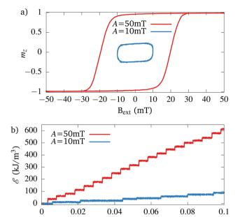
Fig. 5 (a) Hysteresis loops for an ensemble of 10 000 particles, excited with a sinusoidal externally applied magnetic field with amplitudes of 10 mT (blue lines) and 50 mT (red lines). (b) Dissipated heat by a single particle as function of time for 10 periods of the field excitation.
