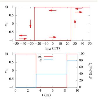
Fig. 4 (a) Hysteresis loop for a single domain particle in an externally applied field parallel with its anisotropy easy axis. (b) The magnetisation along the easy axis  $m_z$  and dissipated energy density  $\mathcal E$  as function of time for a single hysteresis loop. Heat only gets dissipated during the two switching events.
