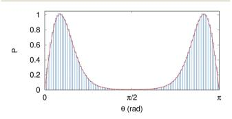
Fig. 2 Probability with maximum normalised to 1, P, to find the magnetisation under an angle  $\theta$  with respect to the anisotropy easy axis, as extracted from simulations (blue bars) and eqn (8) (red line).
