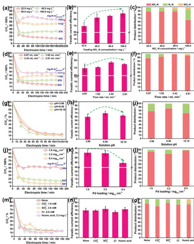
**Fig. 3** Impacts of (a–c) the feeding  $\text{NO}_3^-$ -N concentration, (d–f) flow rate, (g–i) pH, (j–l) Pd loading, and (m–o) co-existing anions and dissolved organics on the  $\text{NO}_3^-$ -N conversion rate, faradaic current efficiency, and product distribution in NRR.
