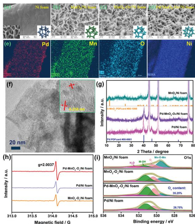
**Fig. 1** Representative SEM images of (a) Ni foam, (b) MnO<sub>2</sub>/Ni foam, (c) MnO<sub>2</sub>-O<sub>v</sub>/Ni foam, and (d) Pd–MnO<sub>2</sub>-O<sub>v</sub>/Ni foam; (e) EDS elemental mapping of Pd, Mn, O, and Ni for Pd–MnO<sub>2</sub>-O<sub>v</sub>/Ni foam; (f) TEM image of Pd/MnO<sub>2</sub>-O<sub>v</sub> nanosheet (inset is the corresponding HRTEM image); (g) XRD patterns of electrodes; (h) EPR spectra and (i) high-resolution O 1s XPS spectra for different electrodes.
