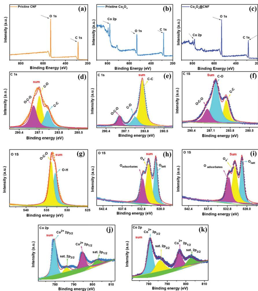
Fig. 3 (a–c) XPS survey spectra of pristine CNF, pristine Co<sub>3</sub>O<sub>4</sub> nanoparticles and 1D Co<sub>3</sub>O<sub>4</sub>@CNF hybrid; (d–f) C 1s binding energy region, (g–i) O 1s binding energy region and (j and k) Co 2p binding energy region for the respective samples.
