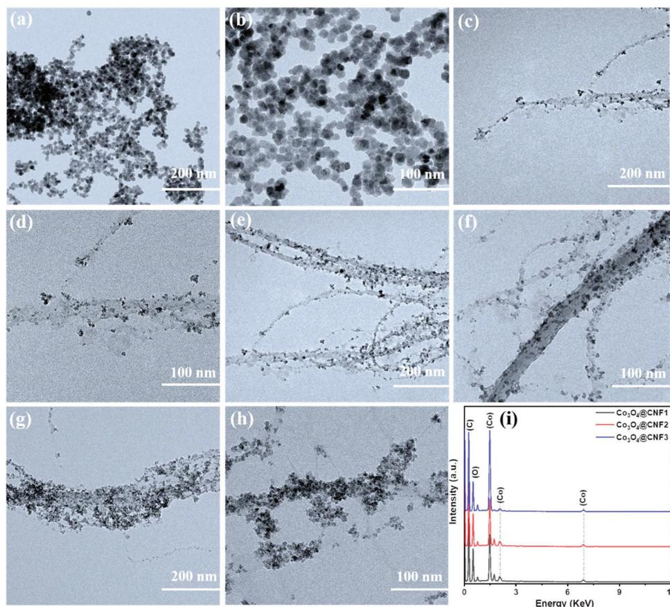
**Fig. 1** TEM images at higher and lower magnification (a and b) of pristine  $\text{Co}_3\text{O}_4$  nanoparticles, (c and d) 1D  $\text{Co}_3\text{O}_4$ @CNF1, (e and f) 1D  $\text{Co}_3\text{O}_4$ @CNF2 and (g and h) 1D  $\text{Co}_3\text{O}_4$ @CNF3 hybrid nanostructure. (i) The elemental spectra of the 1D  $\text{Co}_3\text{O}_4$ @CNF1, 1D  $\text{Co}_3\text{O}_4$ @CNF2 and 1D  $\text{Co}_3\text{O}_4$ @CNF3 hybrid nanostructure.
