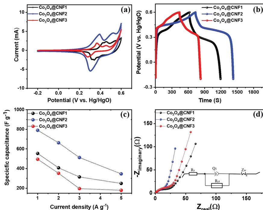
Fig. 4 Electrochemical performance of the three-electrode measurement for the 1D  $Co_3O_4@CNF_x$  hybrid electrodes (where  $x$  means the feeding amount of the  $Co_3O_4$  nanoparticles on the CNF surface): (a) CV curve at  $20 \text{ mV s}^{-1}$  of scan rate, (b) GCD curve of  $1 \text{ A g}^{-1}$  of current density, (c) specific capacitance at the various current densities and (d) electrochemical impedance spectra (EIS).
