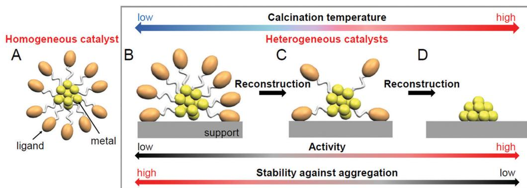
Fig. 1 Categorization of catalysts: (A) homogeneous catalyst (sometimes called quasi-homogeneous catalyst) and (B–D) heterogeneous catalysts. This review discusses heterogeneous catalysts prepared using atomically precise, ligand-protected metal NCs (B–D). Note that calcination induces not only the ligand elimination but also the reconstruction of the metal-core structure.
