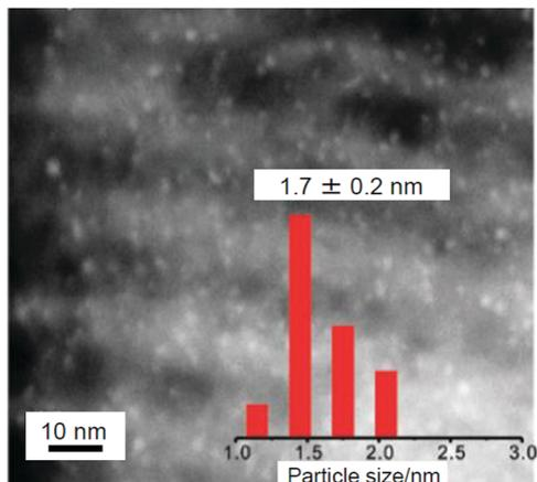
Fig. 20 STEM image of Au<sub>144</sub> NCs (1.1 wt% Au) loaded on CuO-EP-FDU-12 after calcination at 300 °C and size distribution of Au NCs. Reproduced with permission from ref. 234. Copyright 2012 Royal Society of Chemistry.
