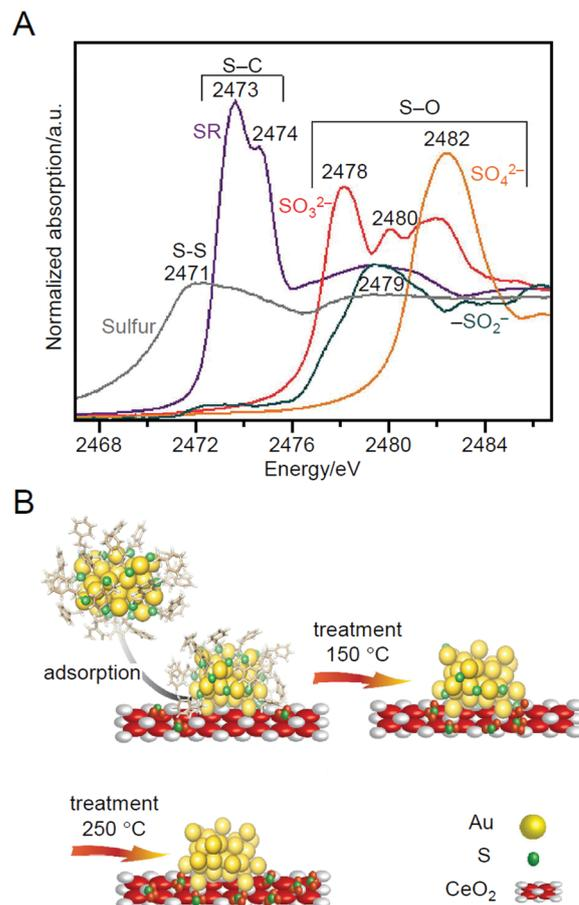
Fig. 10 (A) XANES spectra at S K-edge of different reference materials. (B) Schematic of thiolate ligands evolution upon NC deposition on  $\text{CeO}_2$  and oxidative treatments. Reproduced from ref. 216. Copyright 2018 Wiley-VCH.
