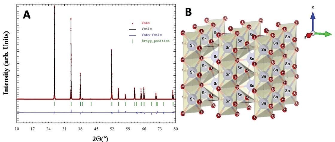
Fig. 3 (A) Rietveld refined XRD pattern of SnO<sub>2</sub>(s). (B) Crystal structure of SnO<sub>2</sub>.
