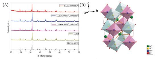
Fig. 1 (A) XRD patterns of LLSO:  $0.005 \text{Mn}^{4+}$ ; LLSO:  $0.097 \text{b}^{3+}$ ,  $0.005 \text{Mn}^{4+}$ ; LLSO:  $0.090 \text{Dy}^{3+}$ ,  $0.005 \text{Mn}^{4+}$  and LLSO host. (B) Crystal structure schematic diagram of La<sub>2</sub>LiSbO<sub>6</sub>.
