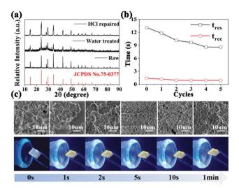
Fig. 4 (a) XRD patterns of  $Cs_2TeCl_6$  before and after the HCl gas treatment. (b) Response and recovery time of the  $Cs_2TeCl_6$ -based device before and after multiple cycles of the HCl gas treatment. (c) SEM images and device physical diagram of the sample with different recovery times (0, 1, 2, 5 s, and 1 min).
