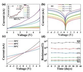
Fig. 3 (a) I-V characteristics of the  $Cs_2TeCl_6$ -based humidity sensor at different ambient environment RH, the inset plot is the current *versus* RH under 5 V bias. (b) Logarithmic representation of the I-V data. (c) I-V characteristics of the  $Cs_2TeCl_6$ -based sensor recorded at different ambient temperatures (30 °C, 40 °C, and 50 °C, respectively). (d) The long-term stability of the sensor in the air under different RH values.
