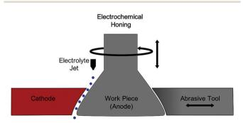
Scheme 3 A schematic of the setup for electrochemical honing as used to achieve controlled surface finish in remanufacturing processes such as for engine valves
