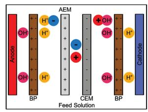
Scheme 6 Simple diagram of the setup for a bipolar membrane electrodialysis, showing the anion exchange membrane (AEM), cation exchange membrane (CEM), and bipolar membranes (BP).
