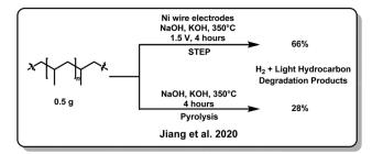
Fig. 11 Solar-thermal-electrochemical process STEP (top) and pyrolysis (bottom) on waste polypropylene. 129
