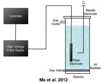
Scheme 10 Schematic representation of the SSP method carried out by Ma et al. and adapted from their work. Licensed under CC BY 3.0.
