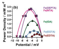
Fig. 2 Power curves for the semi-optimised Fe(ligand) systems, for (a) the polycarboxylate ligands acetate (Fe(Ac)), malonate (Fe(Mal)), and citrate (Fe(Cit)) and (b) the poly-aminocarboxylate ligands IDA (Fe(IDA)), NTA (Fe(NTA)), EDTA (Fe(EDTA)), EGTA (Fe(EGTA)) and DEPTA (Fe(DEPTA).
