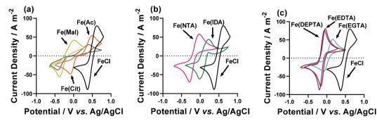
Fig. 4 Cyclic voltammograms of (a) Fe(Ac), Fe(Mal) and Fe(Cit), (b) Fe(IDA) and Fe(NTA) and (c) Fe(EDTA), Fe(EGTA) and Fe(DEPTA) redox couples; all are compared to the parent  $FeCl_{2/3}$  species (i.e. 50 mM  $FeCl_2$  and 50 mM  $FeCl_3$ , in the absence of any ligand). All voltammograms were recorded at an Au working electrode, at a scan rate of 50 mV  $s^{-1}$  and ambient temperature.
