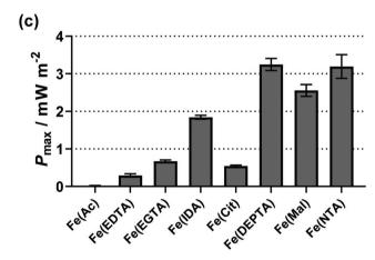
Fig. 3 Bar charts showing (a) the observed Seebeck coefficient ( $S_{\rm e}$ ), (b) the short-circuit current density ( $j_{\rm SC}$ ) and (c) the maximum power density ( $P_{\rm max}$ ) for the semi-optimised Fe(ligand) systems, visually displaying the values in Table 1.
