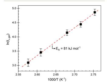
Fig. 2 Plot of the logarithm of the time it took to reach the gel point  $(t_{\alpha,qel})$  vs. the inverse isothermal curing temperature.
