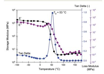
Fig. 5 DMTA data (-100 °C to 180 °C, 1 Hz, 0.1% strain) of cured CBDA-2/ELO thermosets using a fixed COOH/oxirane group-ratio of 0.8 (the symbols are intended to help differentiate the curves and do not represent the sole data points).
