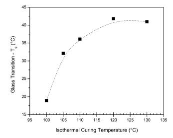
Fig. 3 Obtained  $T_{\rm g}$  of samples cured for 2 h at different isothermal curing temperatures. The  $T_{\rm g}$  was determined immediately after the isothermal curing of the samples by cooling and heating the samples at 10 K min<sup>-1</sup>.
