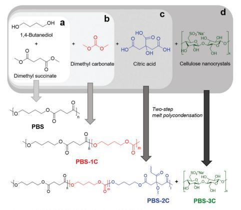
Fig. 1 Scheme for the syntheses of: (a) PBS, (b) PBS-1C, (c) PBS-2C, and (d) PBS-3C.
