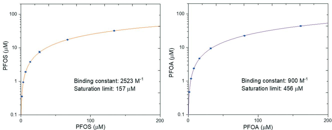
Fig. 3 Fitted binding isotherm of PFOS and PFOA.
