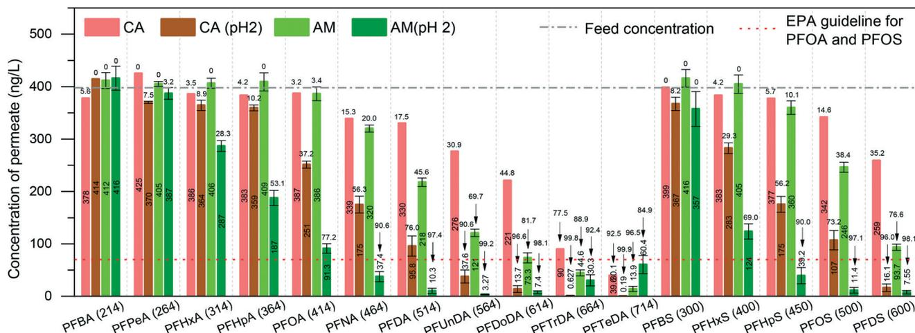
**Fig. 1** Concentrations of PFCAs and PFSAs in the permeate. The pH of the feed is around 7 unless otherwise stated. The number in the brackets is the MW of each compound. The red dashed line stands for EPA guideline for PFOA and PFOS regulation, which is  $70 \text{ ng L}^{-1}$ . The grey dashed line stands for the spike concentration of each PFAS, which is around  $400 \text{ ng L}^{-1}$ . The removal efficiencies (%) are shown above the permeate bars.
