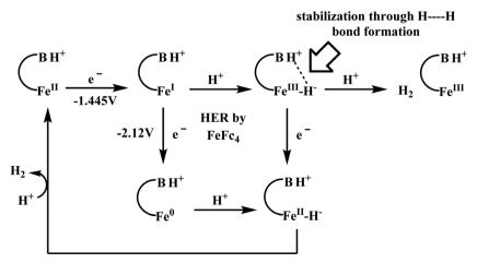
Scheme 38 Probable mechanism of the HER catalysed by Fe porphyrins containing distal triazole basic residues.
