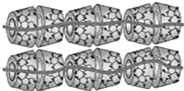
Scheme 11 Conceptual representation of the constrained polymerization of styrene molecules encapsulated within the narrow channels of the \gamma CD host. The scheme has been reproduced from ref. 86 with permission from Wiley-VCH Verlag GmbH.
