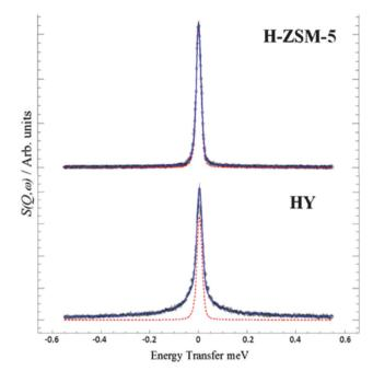
Fig. 10 QENS spectra at 298 K of methanol loaded in zeolites H-ZSM-5 and HY at Q = 0.9 Å, (--) represents the resolution data taken at 5 K. Reprinted from ref. 172 with permission of the Royal Society of Chemistry.
