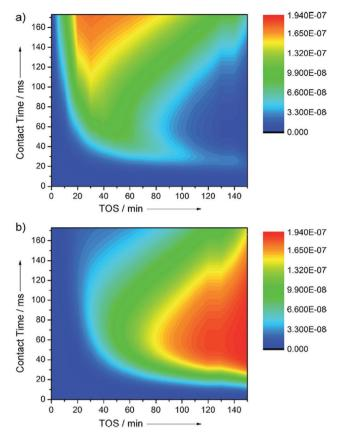
Fig. 2 Formation of (a) aromatic HCP reaction intermediates, and (b) coke, from a kinetic model of the MTO process. The initial progress of hydrocarbon pool intermediates towards the bed inlet with TOS is clearly modelled, as is the formation of coke which spreads towards the outlet and causes the final expansion and deactivation. Reprinted from ref. 22, with permission from Wiley
