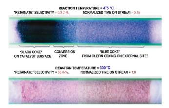
Fig. 1 Photographs of the H-ZSM-5 catalyst bed after methanol conversion at high (above) and low (below) temperature. Reprinted from ref. 19 with permission from Elsevier.
