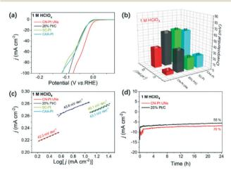
Fig. 5 Comparison of the HER performance of CN-Pt UNs and the other catalysts in 1 M HClO $_4$ : (a) HER polarization curves, (b) overpotentials at 10 mA cm $^{-2}$  and 50 mA cm $^{-2}$ , (c) Tafel curves, and (d) time-dependent current density curves in 1 M HClO $_4$ .
