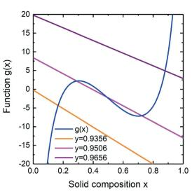
Fig. 3 Illustration of the y(x) selection rule for InGaAs materials system. The blue solid curve is g(x) function; the tilted lines are f(y) + u(y)x calculated for different y and at fixed  $a_{GaAs}/a_{InAs} = 1.3$ .
