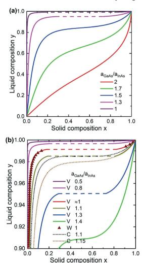
Fig. 4 Liquid-solid composition dependences of InGaAs alloy for different surface energy ratio calculated within the Vegard model (a) and within Vegard (V), Wilemski (W) and convex (C) models (b). Triangles correspond to the Wilemski approach. The solid curves are the Vegard's law case and dots are the convex model with  $\alpha$  = 0.5. The dashed lines correspond to the miscibility gap.
