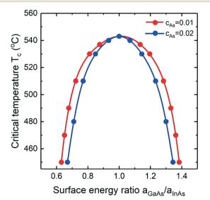
Fig. 7 Critical temperature versus the ratio of binary surface energy terms for InGaAs materials system at fixed As concentration of  $c_{As}$  = 0.01 (red curve) and  $c_{\rm As}$  = 0.02 (blue curve). The dots represent numerical calculations and the solid curves are polynomial fits.
