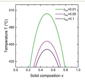
Fig. 6 The miscibility gap in InGaAs alloy at  $a_{GaAs}/a_{InAs}$  = 1.3 for different As concentrations.
