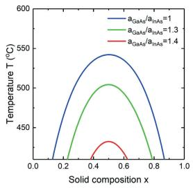
Fig. 5 The miscibility gap in  $In_xGa_{1-x}As$  alloy at  $c_{As} = 0.01$  for different surface energy ratios
