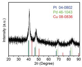
Fig. 1 XRD pattern of the PtPdCu cubic nanoframes.
