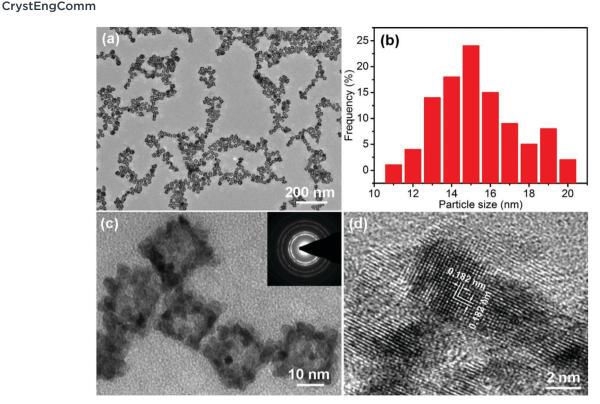
Fig. 3 (a and c) TEM images, (b) size distribution histogram and (d) HRTEM image of the PtPdCu cubic nanoframes, inset in (c) is a SAED pattern of the PtPdCu cubic nanoframes.
