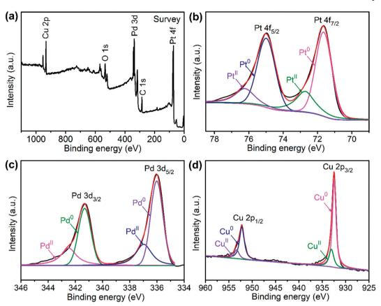
Fig. 2 XPS spectra of the PtPdCu cubic nanoframes: (a) survey scan, (b) Pt 4f, (c) Pd 3d and (d) Cu 2p.
