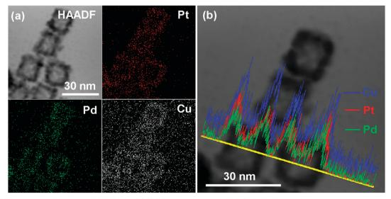
Fig. 4 (a) HAADF and elemental mapping images, and (b) EDS line scan image of the PtPdCu cubic nanoframes.
