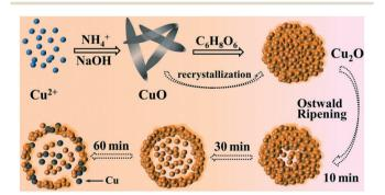
Fig. 5 Schematic diagram of the formation process of Cu<sub>2</sub>O hollow spheres.
