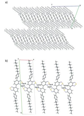
Fig. 2 a) A view of the crystallographic packing of 4 showing the layered arrangement. b) A view of the sheets that form the layer growing along the a direction interacting through chalcogen bonding 2S-2N squares.
