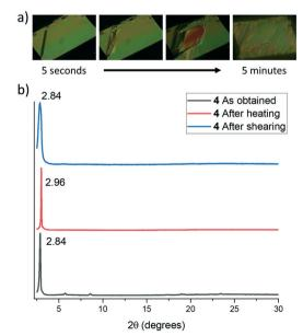
**Fig. 6** a) POM images of the polymorphic transformation occurring on a single crystal at 70 °C. b) Thermal and subsequent mechanochromic polymorphic transformations followed by powder X-ray diffraction pattern changes.
