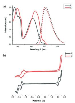
Fig. 1 a) Normalized UV-vis (lines) and fluorescence (dots) spectra of compounds 4-5 in  $CH_2Cl_2$ ,  $c = 5 \times 10^{-6}$  M solutions. b) Cyclic voltammograms of compounds 4-5 at [C] =  $1 \times 10^{-3}$  M recorded at a scan rate of 100 mV s<sup>-1</sup> in CH<sub>2</sub>Cl<sub>2</sub>/0.1 M TBAPF<sub>6</sub> measured versus Ag/ AgCl.
