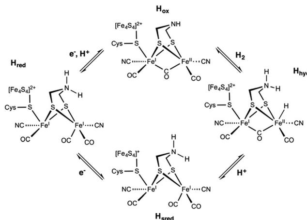
Fig. 11 Postulated reaction mechanism of the [FeFe] hydrogenase involving the H<sub>ox</sub>, H<sub>hyd</sub>, H<sub>red</sub>, and H<sub>sred</sub> states.
