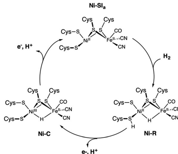
Fig. 10 Proposed catalytic cycle of the [NiFe] hydrogenase involving the Ni–SI<sub>a</sub>, Ni–R, and Ni–C states.
