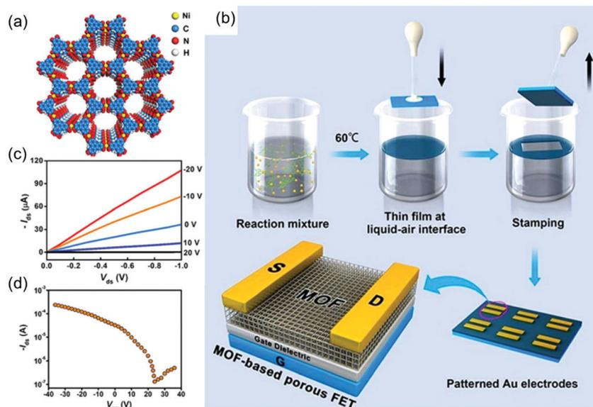
Fig. 15 (a) Schematic structure of semiconducting Ni<sub>3</sub>(HITP)<sub>2</sub>. (b) Schematic illustration of the fabrication of Ni<sub>3</sub>(HITP)<sub>2</sub> film-based porous FETs. (c and d) Output curves and transfer curve for the Ni<sub>3</sub>(HITP)<sub>2</sub>-based FET, respectively. Reproduced with permission from ref. 164. Copyright 2017 American Chemical Society.
