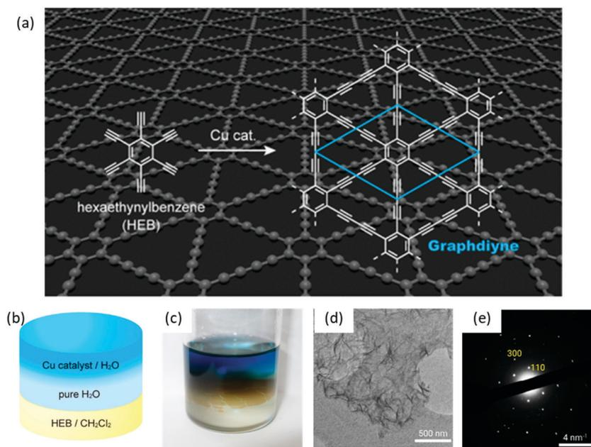
Fig. 4 Liquid/liquid interfacial synthesis and microscopic observations of multilayer GDY. (a) Chemical reaction scheme of hexaethynylbenzene (HEB) to form GDY. (b) Schematic illustration and (c) the photograph of the reaction system. (d) TEM image and (e) SAED pattern of the GDY flakes. Reproduced with permission from ref. 59. Copyright 2017 American Chemical Society.
