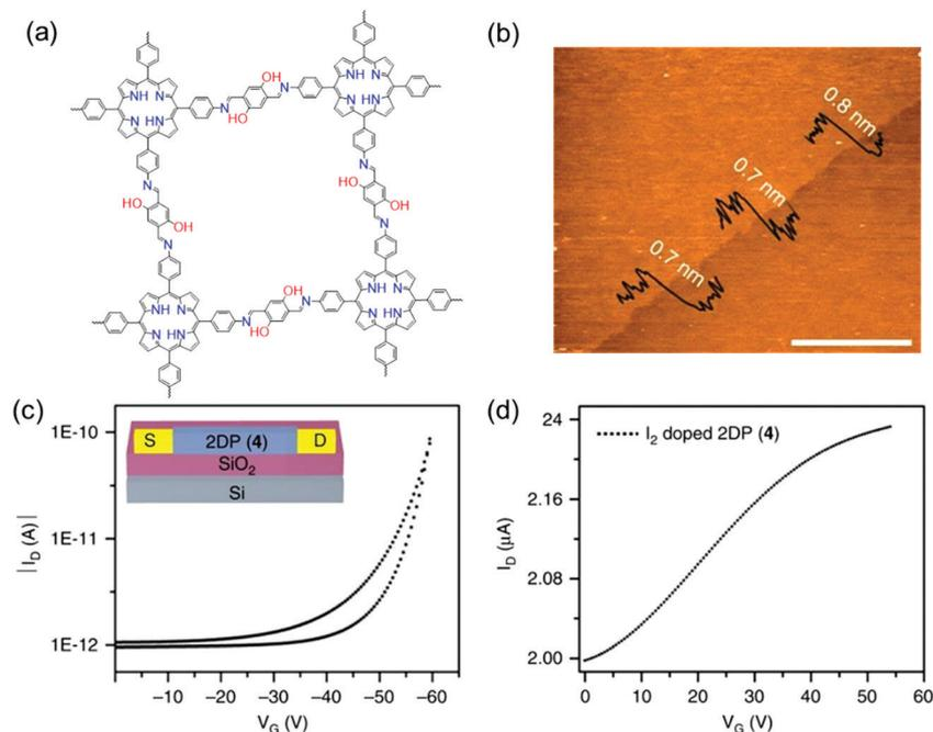
Fig. 10 (a) Chemical structures of 2D polyimine. (b) AFM image of a monolayer. (c) Transfer curve of a thin film transistor at a source to drain voltage of  $-40 \text{ V}$ . (d) Transfer curve of iodine-doped 2D polyimine in the FET device. Reprinted with permission from Macmillan Publishers Ltd: *Nat. Commun.*, ref. 34, copyright 2016.
