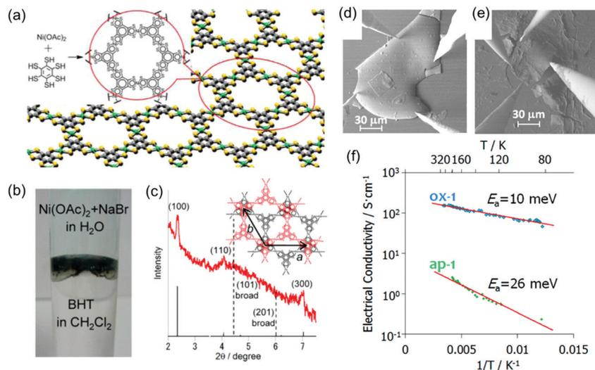
**Fig. 13** (a) Chemical structure of the monolayer HTB-Ni 2D c-MOF. (b) Synthesis of the 2D c-MOF film at the  $\text{CH}_2\text{Cl}_2$ -water interface. (c) XRD of the synthetic film. (d and e) SEM images for the van der Pauw measurement of oxidized and as-prepared HTB-Ni films, respectively. (f) Temperature dependent electrical conductivity. Sample thickness:  $1 \mu\text{m}$ . Reproduced with permission from ref. 31 and 141. Copyright 2013 and 2014 American Chemical Society, respectively.
