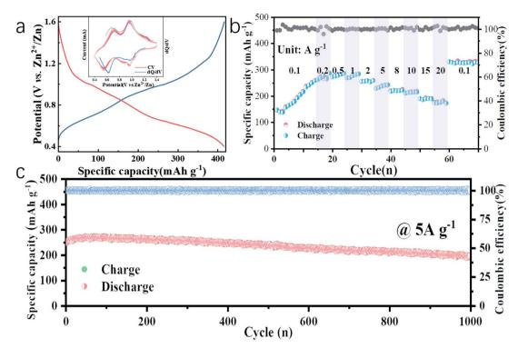
Fig. 2 Electrochemical performance of the Zn// $V_2O_5$ -YS battery: (a) galvanostatic discharge/charge profiles at a current density of 0.1 A g<sup>-1</sup> (inset: the corresponding dQ/dV curve (blue) and CV curves (red)); (b) rate capability; (c) long cycling performance at 5.0 A g<sup>-1</sup>.
