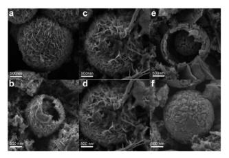
Fig. 6 The ex situ SEM images of the V<sub>2</sub>O<sub>5</sub>-YS cathode at different voltage states (a and b) 1st discharged to 0.98 V (c and d) 1st fully discharged to 0.4 V (e and f) 1st fully charged to 1.6 V.
