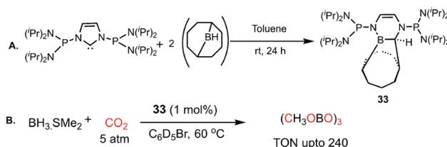
Scheme 7 (A) Preparation of intramolecular P/B FLP system. (B) Catalytic CO<sub>2</sub> reduction using the P/B FLP **33**.
