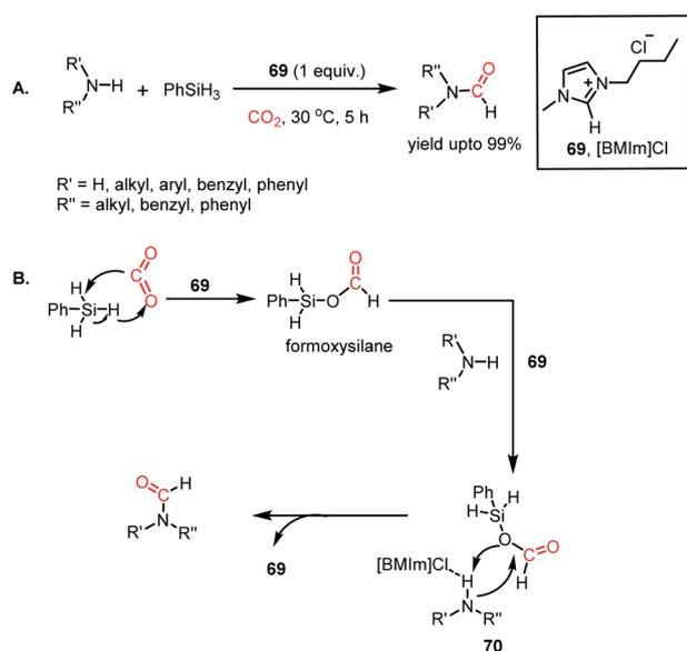
Scheme 24 (A) Ionic liquid (**69**)-mediated amine formylation with CO<sub>2</sub>. (B) Plausible mechanistic steps for amine formylation using **69**.
