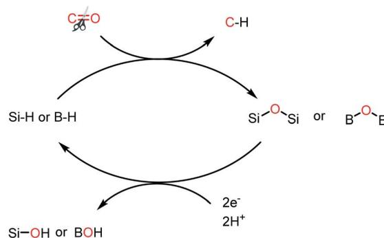
Scheme 36 Use of silane and borane for the reduction of CO<sub>2</sub> will be sustainable if they can be recycled in an energy efficient way.
