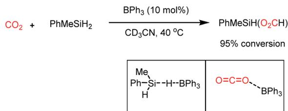
Scheme 16 Selective hydrosilylation of CO<sub>2</sub> into silylformate using a Lewis acid (BPh<sub>3</sub>) as the catalyst.
