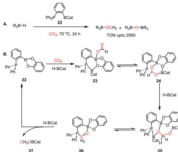
Scheme 5 (A) Catalytic reduction of CO<sub>2</sub> using ambiphilic B/P FLP catalyst. (B) Plausible catalytic cycle using ambiphilic B/P FLP catalyst based on DFT calculation.
