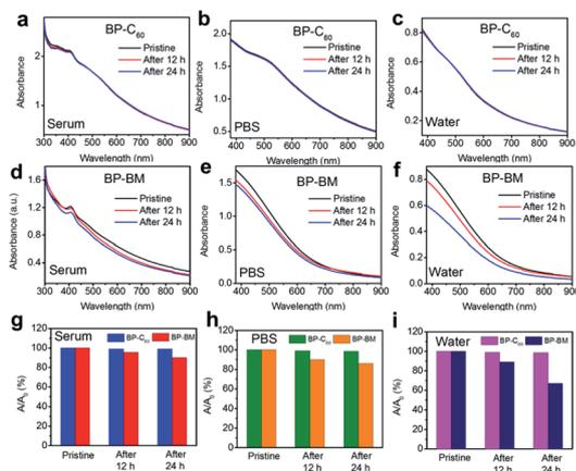
**Fig. 2** Stability of the BP-C<sub>60</sub> hybrid and BP-BM dispersions in serum, PBS and water. UV vis absorption spectra of the BP-C<sub>60</sub> hybrid (a–c) and BP-BM (d–f) dispersed in serum (a and d), PBS (b and e) and water (c and f) after standing for 12 and 24 hours. Variation of the absorption ratios ( $A/A_0$ ) at 460 nm of the BP-C<sub>60</sub> hybrid and BP-BM dispersed in serum (g), PBS (h) and water (i) after standing for 12 and 24 hours.
