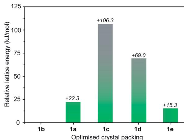
Fig. 4 Energy landscape of the experimentally observed phases of **1a–e**, relative to **1b**. The calculated lattice energies are based on DFT optimisation including dispersion interactions with apical paddlewheel solvents omitted.
