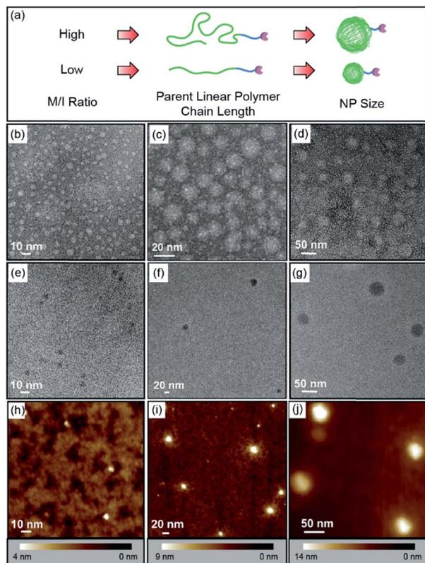
Fig. 3 (a) Illustration of the synthesis of different-sized monovalent ONP-N<sub>3</sub>. (b–d) Negatively stained TEM images of ONP<sup>S/M/L</sup>. (e–g) Brightfield TEM images of ONP<sup>S/M/L</sup> using ultrathin carbon layer grid. (h–j) AFM images of ONP<sup>S/M/L</sup> using PeakForce Tapping mode under ambient condition.
