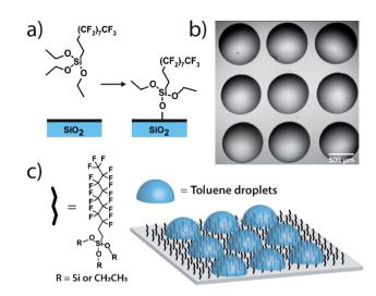
Fig. 1 Surface functionalization for droplet immobilization: (a) deposition of perfluorodecyltriethoxysilane. (b) Bright field image of a  $3 \times 3$ array of toluene droplets immobilized on a glass coverslip, surrounded by an aqueous continuous phase. (c) The prepared hydrophobic fluorinated glass surface has a high relative affinity for organic solvent, allowing droplet array immobilization.
