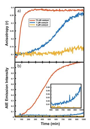
Fig. 5 Monitoring norbornene/toluene droplets at different catalyst concentrations: (a) anisotropy response curves and (b) AIE response curves in droplets containing 70  $\mu\text{M}$  (red), 7  $\mu\text{M}$  (blue), and 0  $\mu\text{M}$  (yellow) Grubbs Gen II catalyst. Inset shows late time intensity dynamics.
