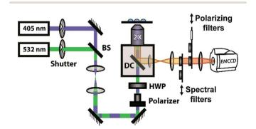
Fig. 2 Optical setup for fluorescence measurements. Synchronized shutters and sliding mounts allow for alternating excitation with 405 nm and 532 nm light for the two probe monomers and collection through appropriate spectral and polarizing filters. BS: beamsplitter; HWP: half-wave plate; DC: dichroic.
