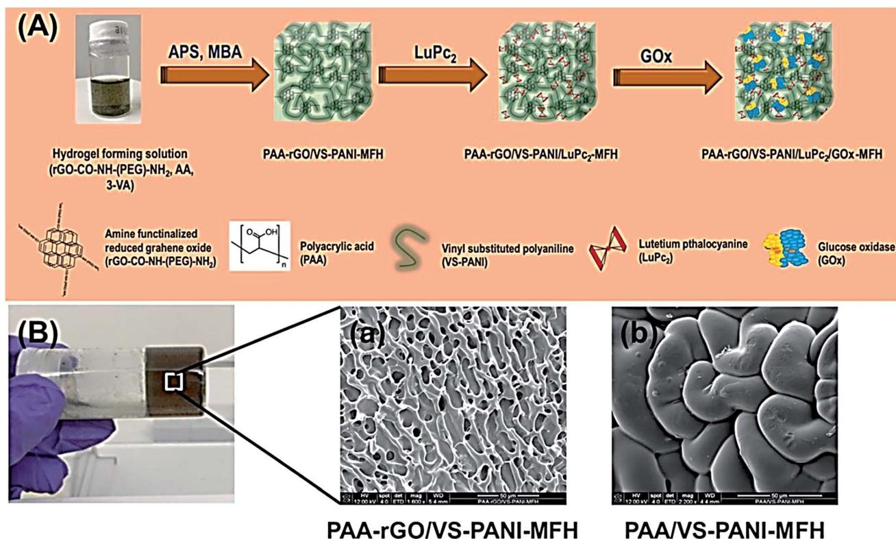
Fig. 9 (A) The PAA-rGO/VS-PANI/LuPc<sub>2</sub>/GO<sub>x</sub>-MFH synthesis procedure. (B) SEM images of (a) PAA-rGO/VS-PANI-MFH, and (b) PAA/VS-PANI-MFH. Reproduced with permission from ref. 90. Copyright 2017 Elsevier.
