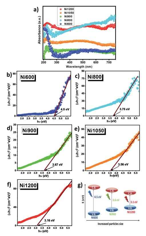
Fig. 7 (a) UV-vis spectra at room temperature of NZFAO samples annealed at different temperature. (b-f) Variation of  $(\alpha h \nu)^2$  versus photon energy  $h\nu$  plot for band gap calculation of annealed Ni<sub>0.6</sub>Zn<sub>0.4</sub>Al<sub>0.5</sub>Fe<sub>1.5</sub>O<sub>4</sub> samples. (g) Schematic band structure obtained according to the obtained results.
