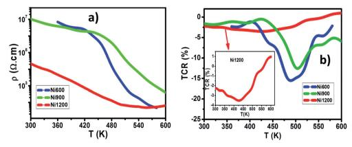
Fig. 12 (a) The temperature dependence of direct-current resistivity for Ni600, Ni900 and Ni1200 samples. (b) The TCR as a function of temperature for Ni600, Ni900, and Ni1200.
