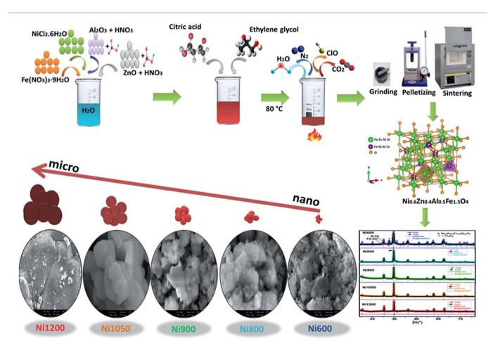
Fig. 1 Chemical reaction of Ni<sub>0.6</sub>Zn<sub>0.4</sub>Al<sub>0.5</sub>Fe<sub>1.5</sub>O<sub>4</sub> synthesized by sol-gel method
