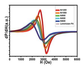
Fig. 11 First derivative (dP/dH vs. H) of resonance signals of different annealing temperatures NZFAO nanoferrites.
