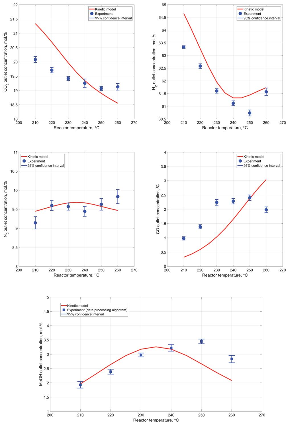
Fig. 8 (a). Dependence of the outlet  $\text{CO}_2$  concentration from the reactor temperature. (b) Dependence of the outlet  $\text{H}_2$  concentration from the reactor temperature. (c). Dependence of the outlet  $\text{N}_2$  concentration from the reactor temperature. (d). Dependence of the outlet CO concentration from the reactor temperature.
