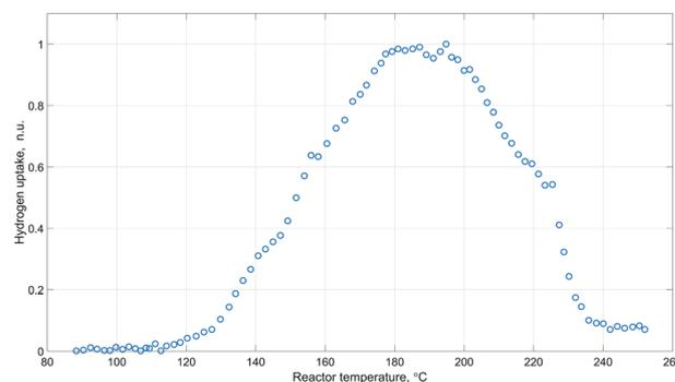
Fig. 5 Hydrogen uptake (normalized units) as a function of reactor temperature during catalyst activation (ambient pressure; inlet gas flowrate 250 N ml min<sup>-1</sup>; inlet gas composition: 20 mol% H<sub>2</sub> and 80 mol% N<sub>2</sub>).
