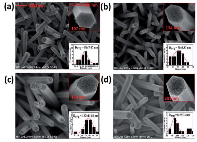
Fig. 1 FESEM analysis of the top-down view of the (a) undoped ZnO NWs, (b) Bi:ZnO-1% NWs, (c) Bi:ZnO-3% NWs, and (d) Bi:ZnO-5% NWs. The top and bottom insets in (a) – (d) show the high-resolution image of a single nanowire and the average diameter measurements for the respective sample.
