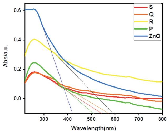
Fig. 3 UV-VIS-DRS spectrum of ZnO and ZnO/rGO composites.
