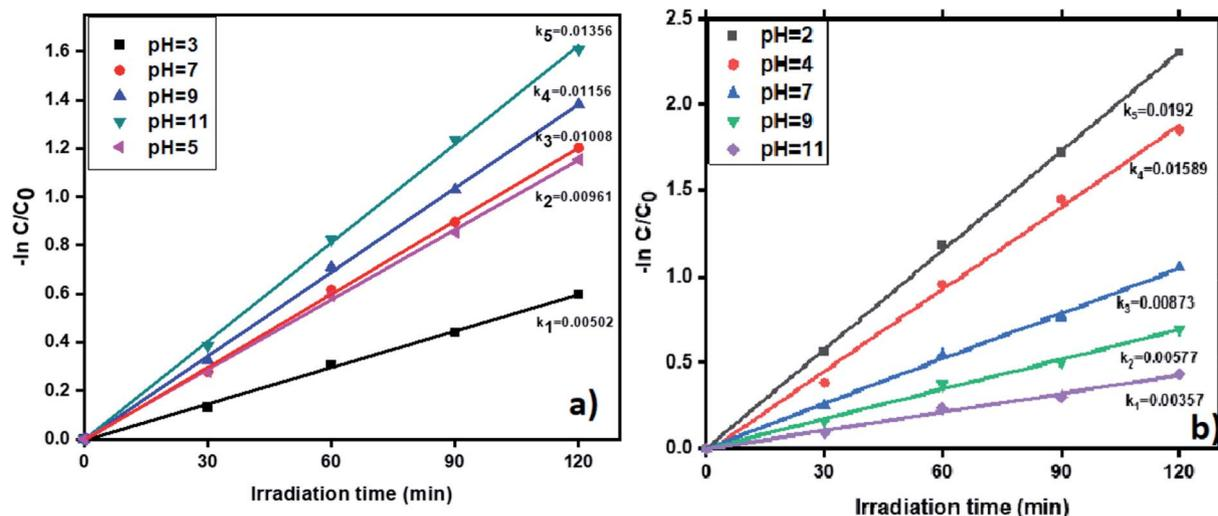
Fig. 11 The kinetic data for effect of pH on (a) TC and (b) Cr(vi) with photocatalyst R (2 h of irradiation time, 50 mg L<sup>-1</sup> of catalyst, 20 ppm of TC, 20 ppm of Cr(vi)).
