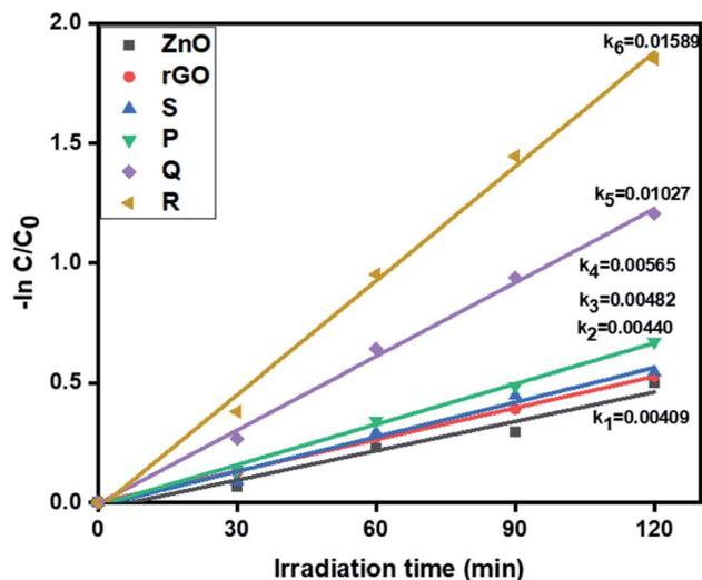
Fig. 7 The kinetic data of ZnO, rGO and ZnO/rGO composites for Cr(vi) reduction (120 min of irradiation time, 50 mg L<sup>-1</sup> of catalyst, 20 ppm of Cr(vi)).
