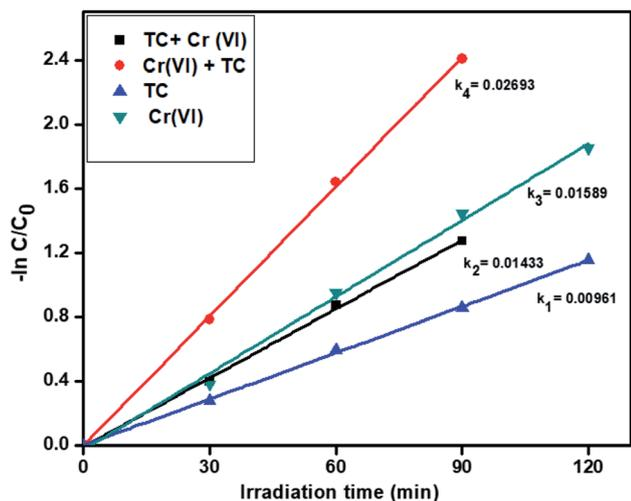
Fig. 8 The kinetics data for the simultaneous removal of TC oxidation and Cr(vi) reduction (120 min of irradiation time, 50 mg L<sup>-1</sup> of catalyst R, 20 ppm of TC, 20 ppm of Cr(vi), pH = 5 of TC, pH = 4 of Cr(vi)).
