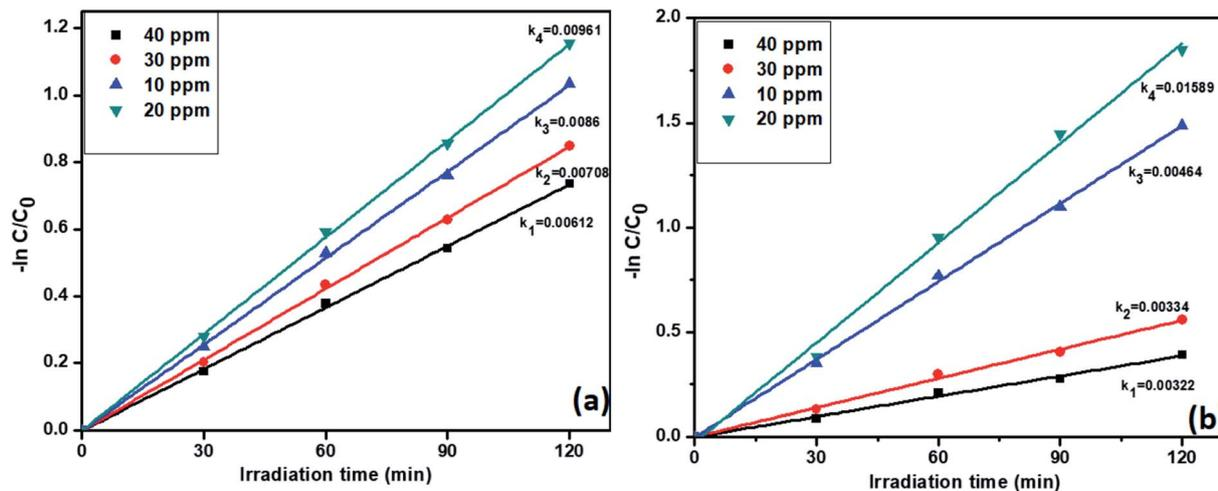
Fig. 9 The kinetic data for the effect of concentration on (a) TC oxidation and (b) Cr(VI) reduction with photocatalyst R (2 h of irradiation time, 50 mg L<sup>-1</sup> of catalyst, pH = 5 of TC, pH = 4 of Cr(VI)).
