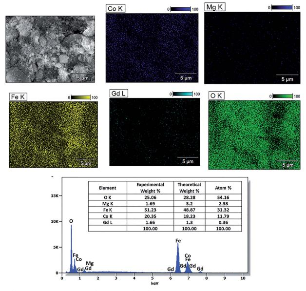
Fig. 6 EDS spectrum and elemental maps of  $Co_{0.7}Mg_{0.3}Fe_{1.98}Gd_{0.02}O_4$  and the corresponding elemental composition.
