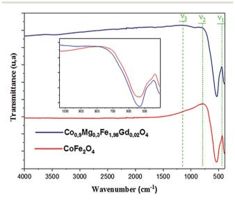
Fig. 4 FTIR spectra of samples Co<sub>0.7</sub>Mg<sub>0.3</sub>Fe<sub>1.98</sub>Gd<sub>0.02</sub>O<sub>4</sub> and CoFe<sub>2</sub>O<sub>4</sub>.
