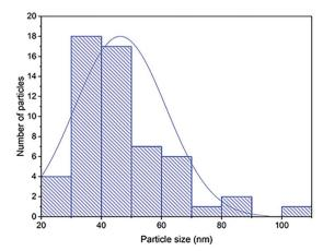
Fig. 5 SEM image of Co<sub>0.7</sub>Mg<sub>0.3</sub>Fe<sub>1.98</sub>Gd<sub>0.02</sub>O<sub>4</sub> nanoparticles and the corresponding particle size distribution.
