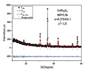
Fig. 2 Typical Rietveld-refined XRD pattern for the CoFe<sub>2</sub>O<sub>4</sub> sample.
