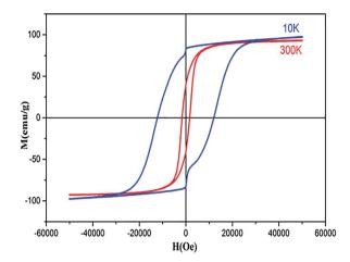
Fig. 7 Hysteresis loops of sample Co<sub>0.7</sub>Mg<sub>0.3</sub>Fe<sub>1.98</sub>Gd<sub>0.02</sub>O<sub>4</sub>.
